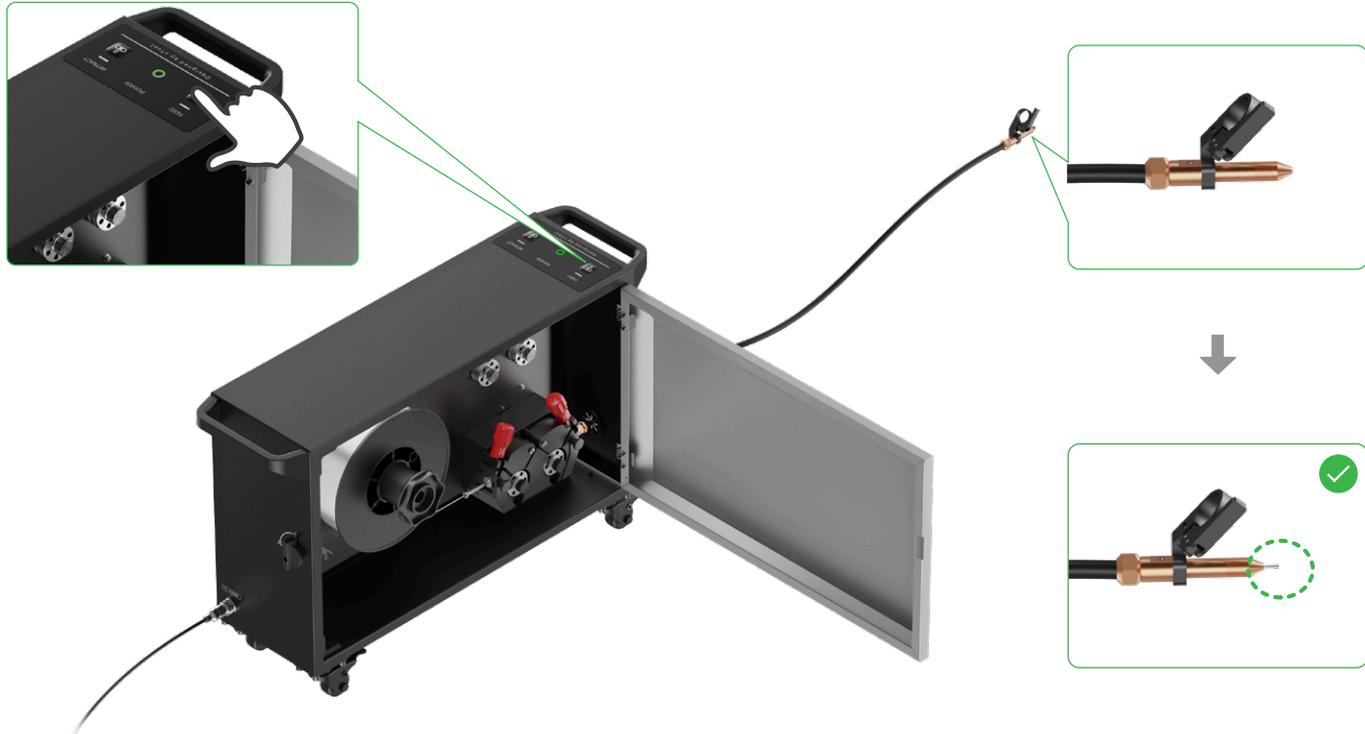
The diagram illustrates the process of inserting the wire nozzle. An inset shows a hand pressing the wire feed button on the top of the unit. The main view shows the unit with its front panel open, revealing the internal wire spool and guide. A callout shows the nozzle being inserted into the end of the wire guide tube. A final callout shows the nozzle fully inserted, marked with a green checkmark.
